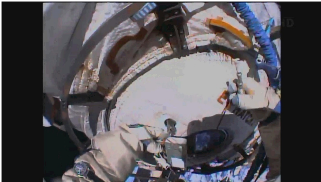
Figure 1. Illuminator of the ISS from which samples of cosmic dust were aseptically recovered
