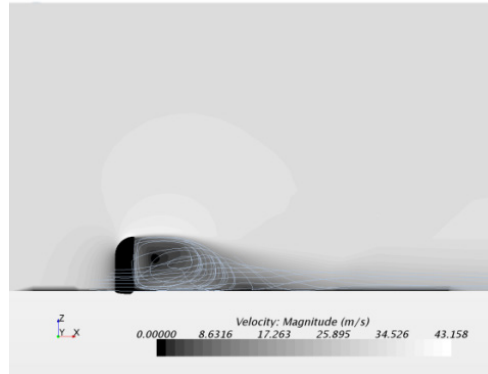
Figure 4-7. The second section average velocity streamline diagram at 3mm of guide bar height
