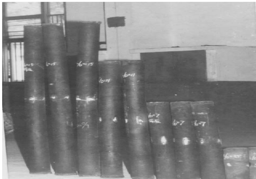
Figure 2. Experimental samples, slender tubes shown after completion of testing
